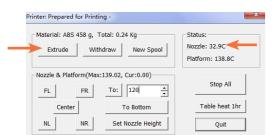
When the printing temperature is reached, the printer will buzz and gently push the filament into the print head until it extrudes at the nozzle.
