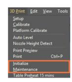
8 Choose "3D Print" - "Autolevel". The autoleveling probe will be released and make its measurements . After printers completes autoleveling, the nozzle height detection process will be initiated automatically.
